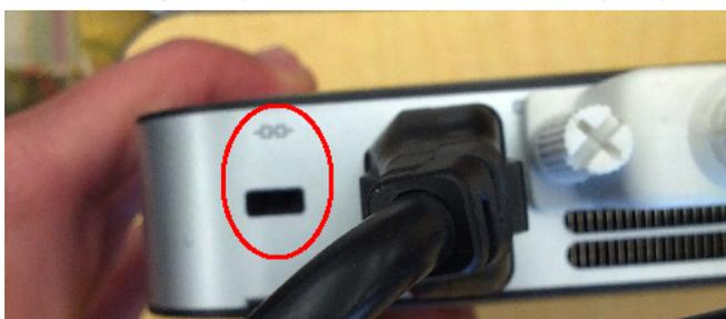
3. Gently move the switch held within the lock port away from the power port using a paper clip or a pin. Moving the switch to this position puts the Chromebox into Developer mode.
