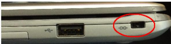
3. Gently move the switch held within the lock port to the right (away from the USB port and towards the monitor) using a paper clip or a pin. Moving the switch to this position puts the Chromebook into Developer mode.
