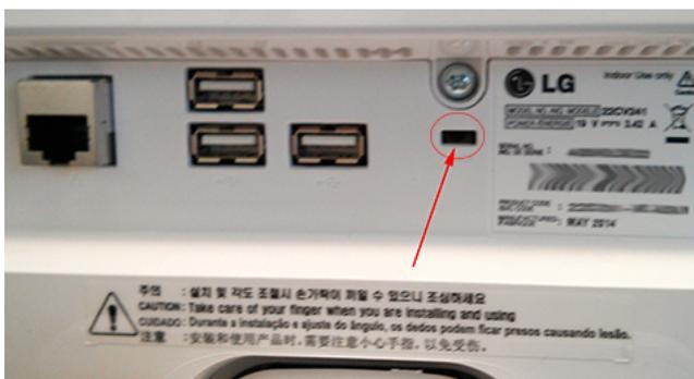
3. Press down the recovery button with a paperclip while turning on the device.
