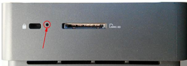
3. Press down the recovery button with a paperclip while turning on the device.
